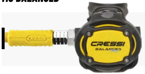
It is a pneumatically balanced valve designed with a Venturi effect adjustment switch, Cressi's patented elliptical membrane diaphragm, and a patented low-friction lever. The Octopus regulator air delivery system without an injector has an internal heat exchange, a cam-lock system to open
