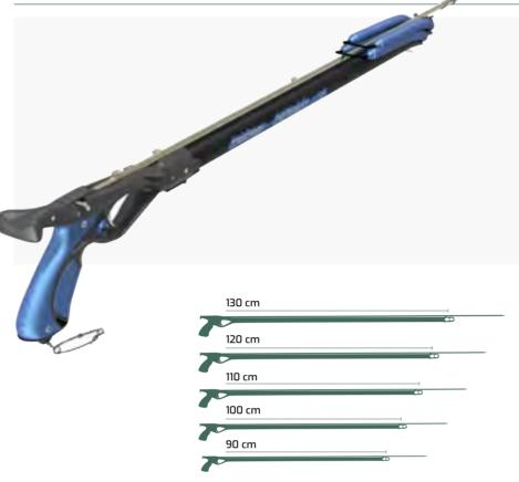
Anticorodal black frame with integrated spear guide, grip made of engineering plastic reinforced with glass fibre, interchangeable high or low soft sternal support. Ultra-light triggering case with trigger, release mechanism and line ring on the side in AISI 316, machined from solid with a CNC process. The shock absorber makes silent the release of the shaft. Reversible side-safety mechanism. Reinforced reel with steel pin buckle.
